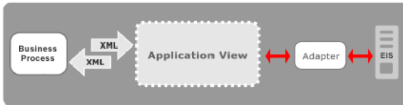
Figure 1-1 Application View in an Integration Solution
