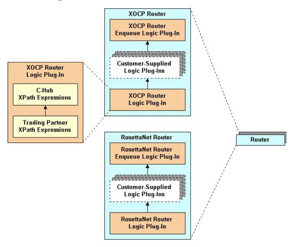
The following figure provides a detailed look at the filter. The filter consists of a protocol-specific filter for each business protocol that WebLogic Collaborate supports.
