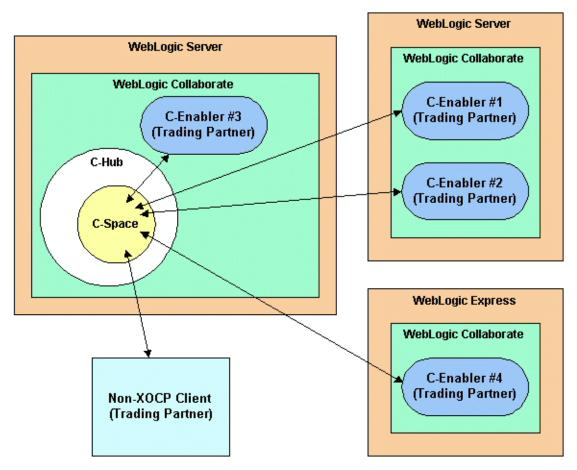
Figure 1-1 Architecture of a Possible WebLogic Collaborate Configuration
