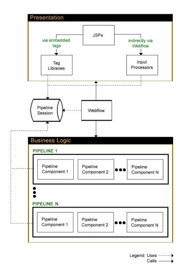
Figure 1-1 Webflow and Pipeline High-level Architecture
