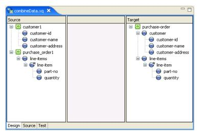
8. Create links between the following source and target elements by dragging elements from the **Source** pane to the **Target** pane.
