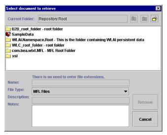
In the Select document to retrieve dialog box, double-click a folder to view its contents, or click the icon to the left of the Current Folder text box to navigate back to the parent folder. Document names and descriptions are displayed to assist in selection. For detailed information about using this dialog box, see "Using the Repository Retrieve and Store Dialog Boxes" on page 5-9.
