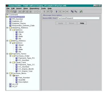
The structure of the binary data is defined in the navigation tree through a combination of fields and groups that match the target data.
