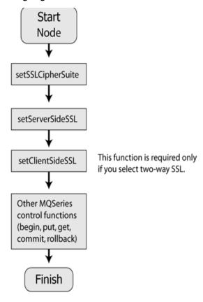
Figure 11-1 Example: Configuring SSL Within a Workflow
