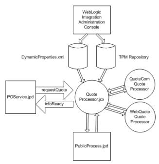
To achieve the required dynamic binding to the target service, the business process defined in POService.jpd uses a Service Broker control, QuoteProcessor.jcx, to call the quote service. Since the target is dynamically specified, the @jc:location tag is not used. The Service Broker control is defined by the following JCX file:
