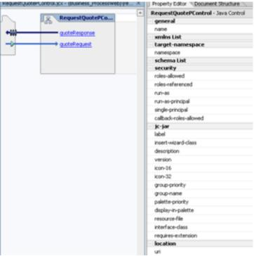
The location of the Process control is displayed in the **location** section of the **Property Editor**, in the **uri** field. The location is not an actual HTTP address, though it may appear that it is. The uri actually displays the location of the object within the Java Naming and Directory Interface (JNDI) tree.
