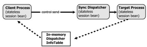
Figure 1-5 Process Control Used for a Synchronous Dispatch
