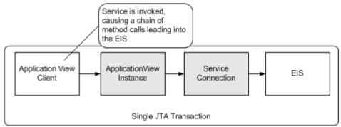
In a synchronous service invocation, a client (for example, a business process) calls the application view (for example, as a control in the business process). The application view calls the adapter using a synchronous Common Client Interface (CCI) request. The service adapter is a J2EE-CA service adapter that actually processes the request.
