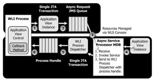
Figure 1-13 Asynchronous Service Invocations—WebLogic Integration Process Client
