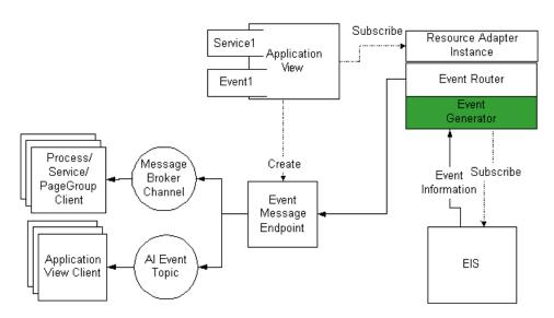
Figure 7-1 Event Connections in a Run-time Environment
