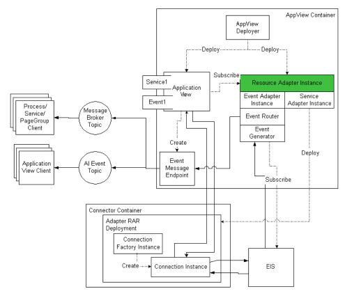
Figure 8-1 Resource Adapters in a Run-time Environment
