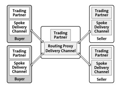
Figure 4-4 Hub-and-Spoke Configuration
