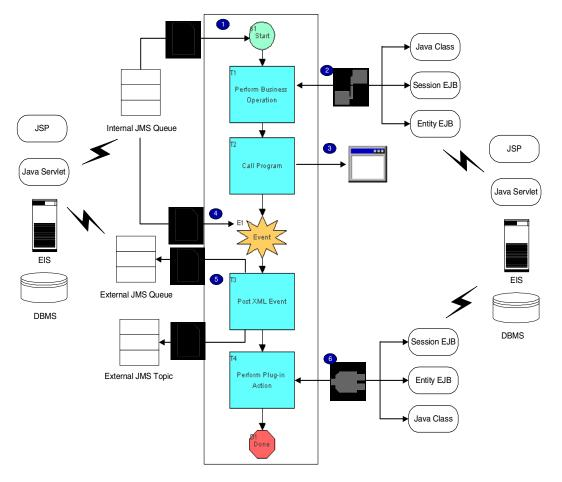
Figure 1-4 Integrating External Components and Applications
