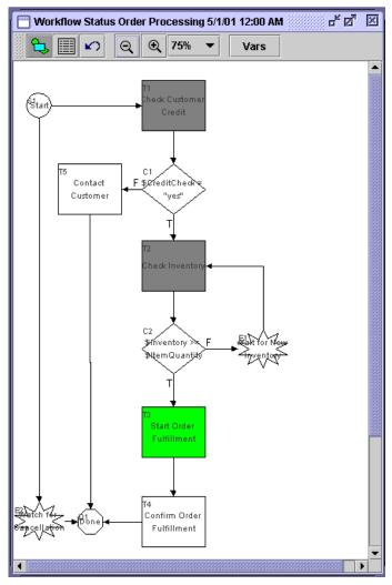
Figure 10-2 Workflow Status Window: Flowchart View
