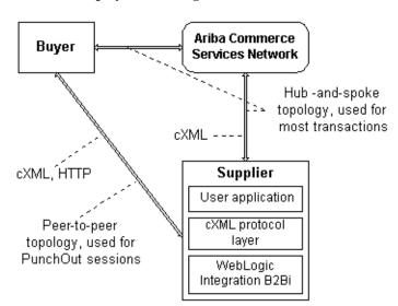
Figure 2-1 cXML Deployment Configurations
