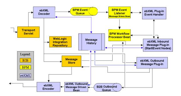
Figure 1-1 WebLogic Integration ebXML Architecture
