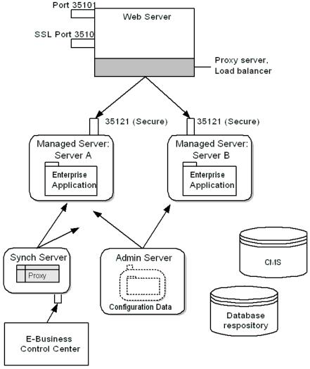
Figure 6-1 Components of a Cluster
