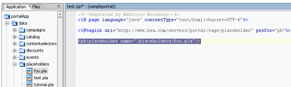
Figure 4-1 The two parts of a placeholder: a placeholder file and a JSP tag
