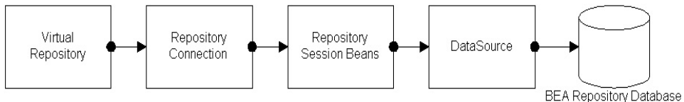
Figure 1-1 Architecture of a Database-based BEA Repository
