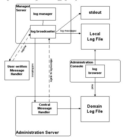
Figure 6-1 WebLogic Server Logging Subsystem
