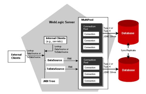
Figure 16-1 JDBC Components in WebLogic Server
