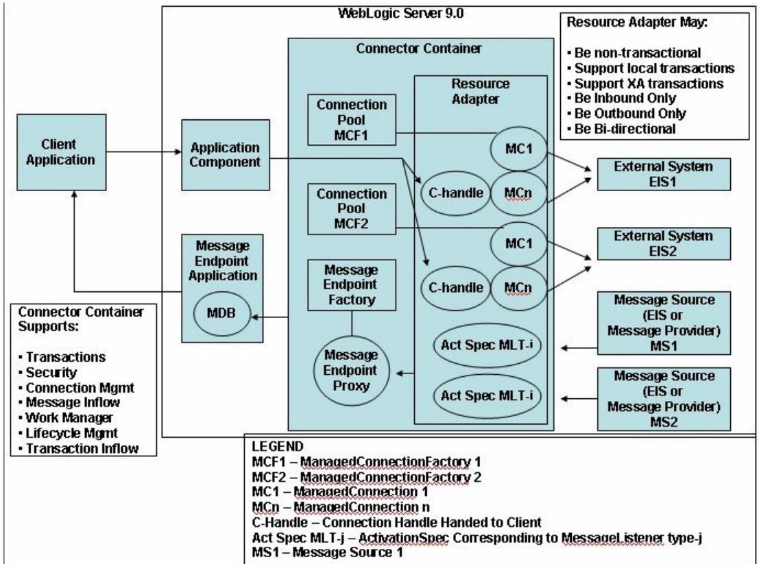
The connector architecture shown in [Figure 2-1, “Connector Architecture Overview,”](#) on [page 2-5](#) demonstrates a bi-directional resource adapter. The following components are used in outbound connection operations:
