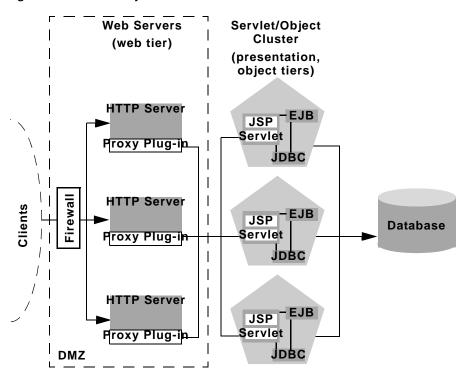
Figure 9-4 Two-Tier Proxy Architecture
