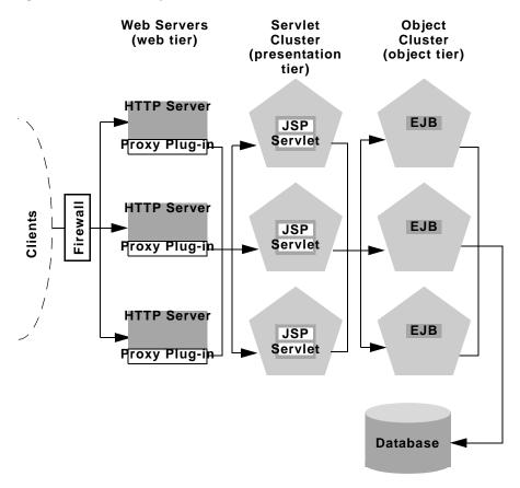
Figure 9-5 Multi-Tier Proxy Architecture
