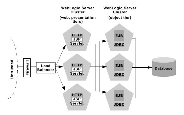
Figure 9-2 Recommended Multi-Tier Architecture
