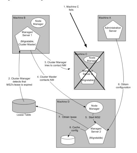
Figure 7-2 Automatic Migration of a Failed Server
