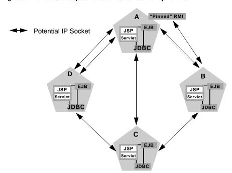
Figure 3-3 Non-Clustered Objects Increase Potential Socket Requirements
