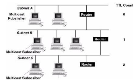
Figure 4-8 Multicast TTL Example
