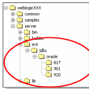
Figure 5-1 Directory Structure for JDBC Drivers Installed with WebLogic Server
