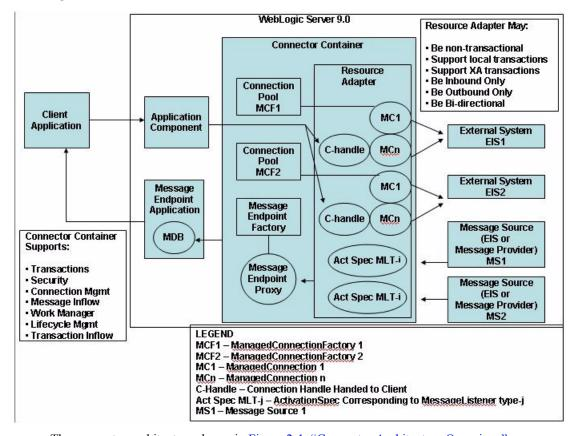
Figure 2-1 Connector Architecture Overview
