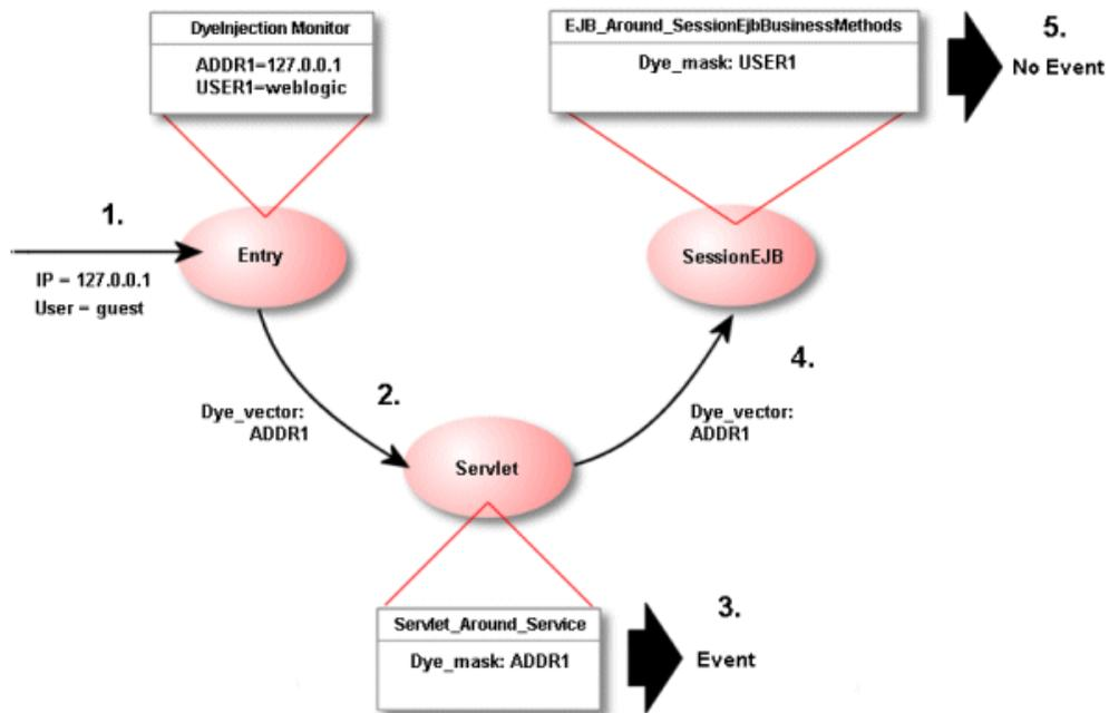
1. A request initiated by user `guest` from IP address `127.0.0.1` enters the system. The user `guest` does not match the value for `USER1` in the `DyeInjection` monitor, so the request is *not* dyed with the dye vector `USER1`. The originating IP address (`127.0.0.1`) matches the value for `ADDR1` defined in the `DyeInjection` monitor, so the request *is* dyed with the dye vector `ADDR1`.
