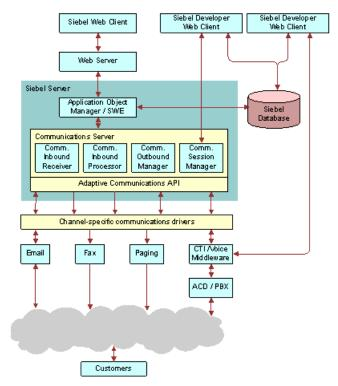
Figure 1. Architecture of Communications Infrastructure
