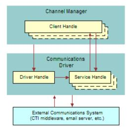
Figure 3. Adaptive Communications Architecture
