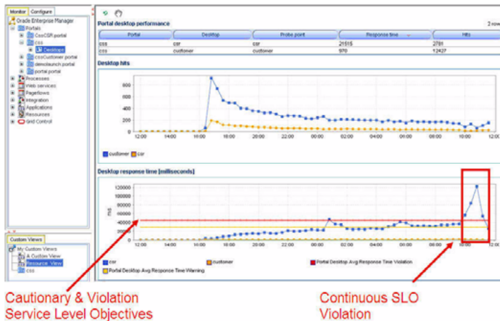
Figure 10-19: Visually Identify SLO Violation
