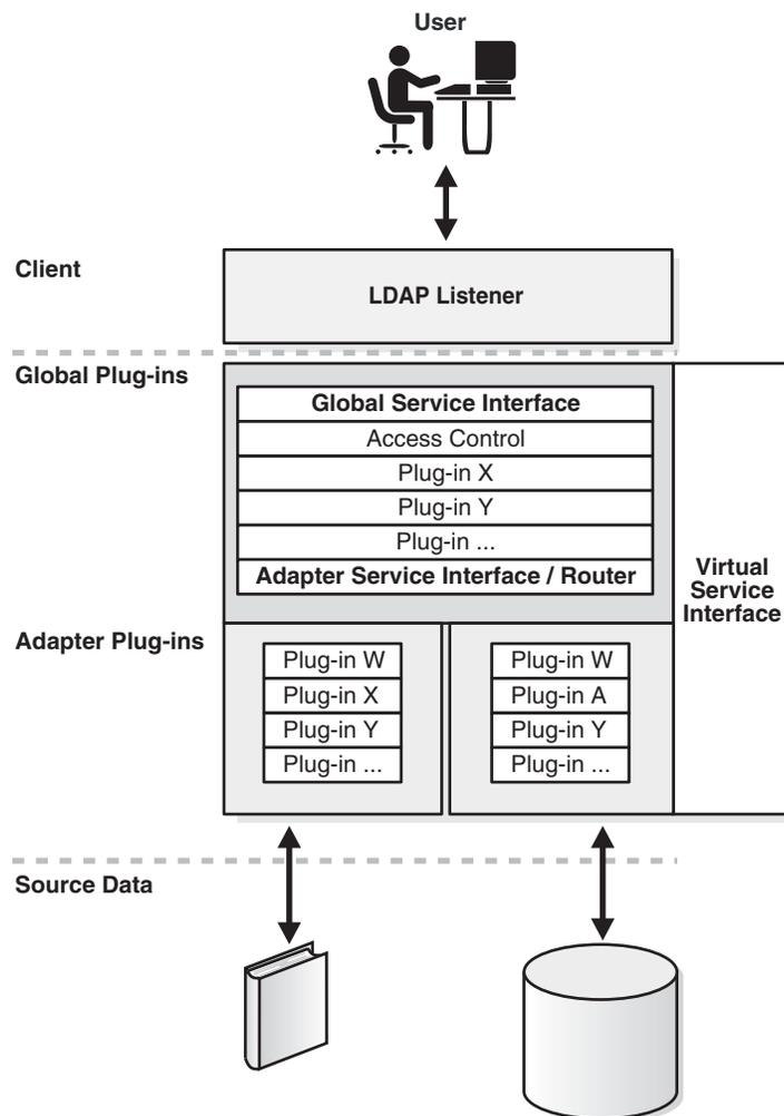
Plug-ins are arranged to form chains. When Oracle Virtual Directory receives a request, the request passes through Oracle Virtual Directory in the following sequence (as shown in [Figure 4-1](#)):
