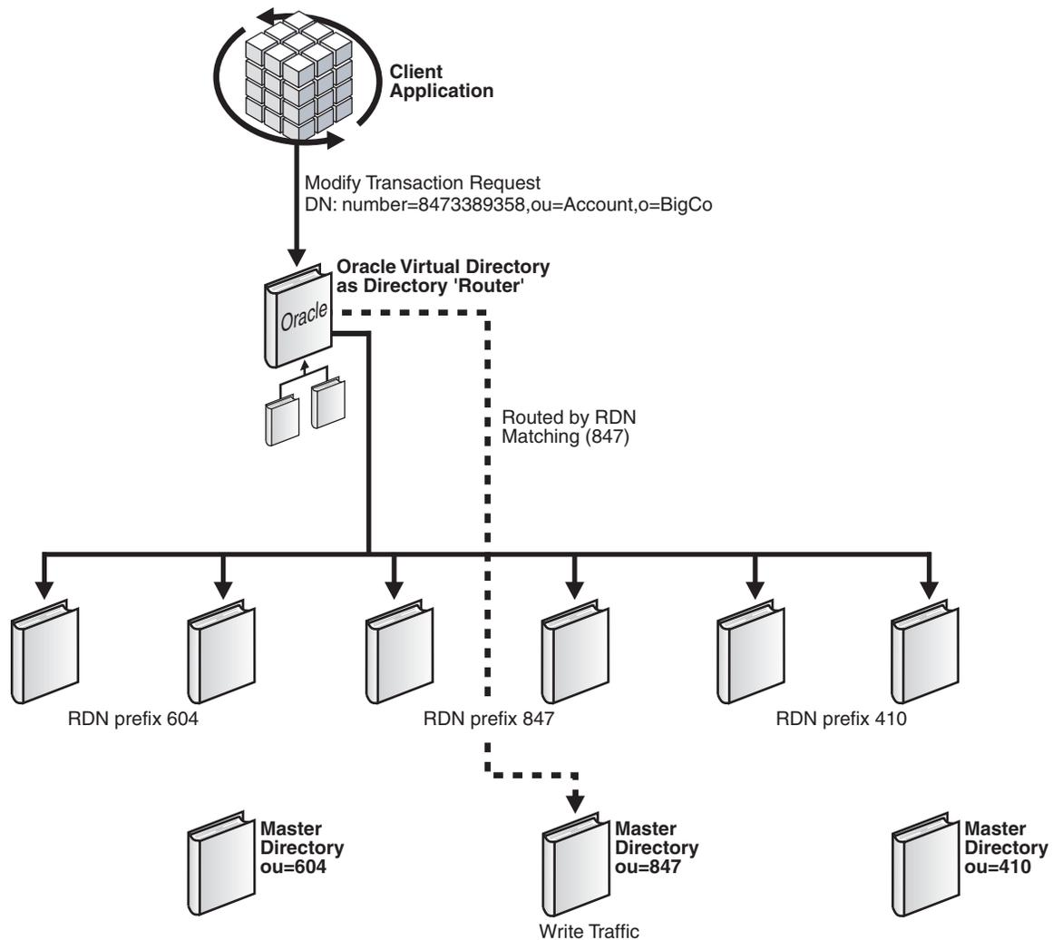
In this case, a routing plug-in mechanism can be used to supplement standard routing features. The intent of the plug-in is to allow you to describe the criteria under which the data will be separated. In order to do this, the criteria selected must ideally be available within every transaction, either in the DN or the filters and base.
