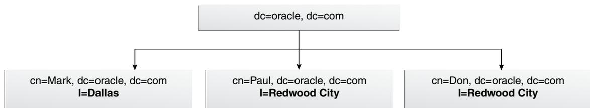
Figure 4-5 shows an example of how the DynamicTree plug-in, with the parentEntryType parameter set to 0 and the attributeName parameter set to l, creates a layered hierarchy in Oracle Virtual Directory based on the l attribute value in the source directory shown in Figure 4-4.
