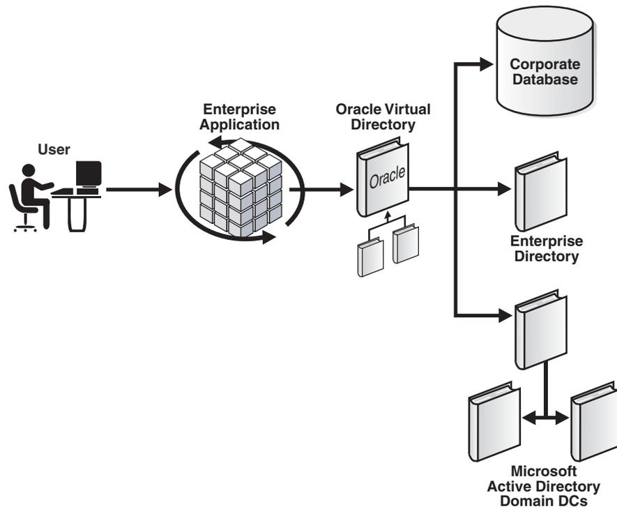
Oracle Virtual Directory hides the complexity of data location, format, and protocol from client applications, similar to a TCP/IP Internet network design based on switches and routers. Switches and routers handle the details of how to establish connections and protocols between different addresses on the network. Oracle Virtual Directory makes many directories appear to be one local repository in much the same way that routers make the entire world appear like it's on your local network.
