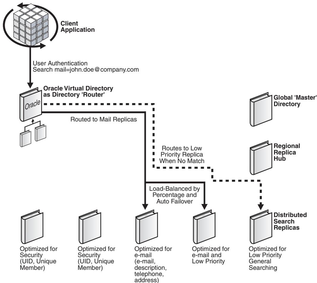
Figure 1–6 shows a typical request where that application is looking to locate a user-distinguished name by searching on UID. Oracle Virtual Directory recognizes the search filter and routes the request to the appropriate directory replicas. Notice that Oracle Virtual Directory can select from multiple nodes and provide load balancing between the nodes, allowing it to spread load across multiple nodes and ensure fault tolerance by not having to rely on any single node.
