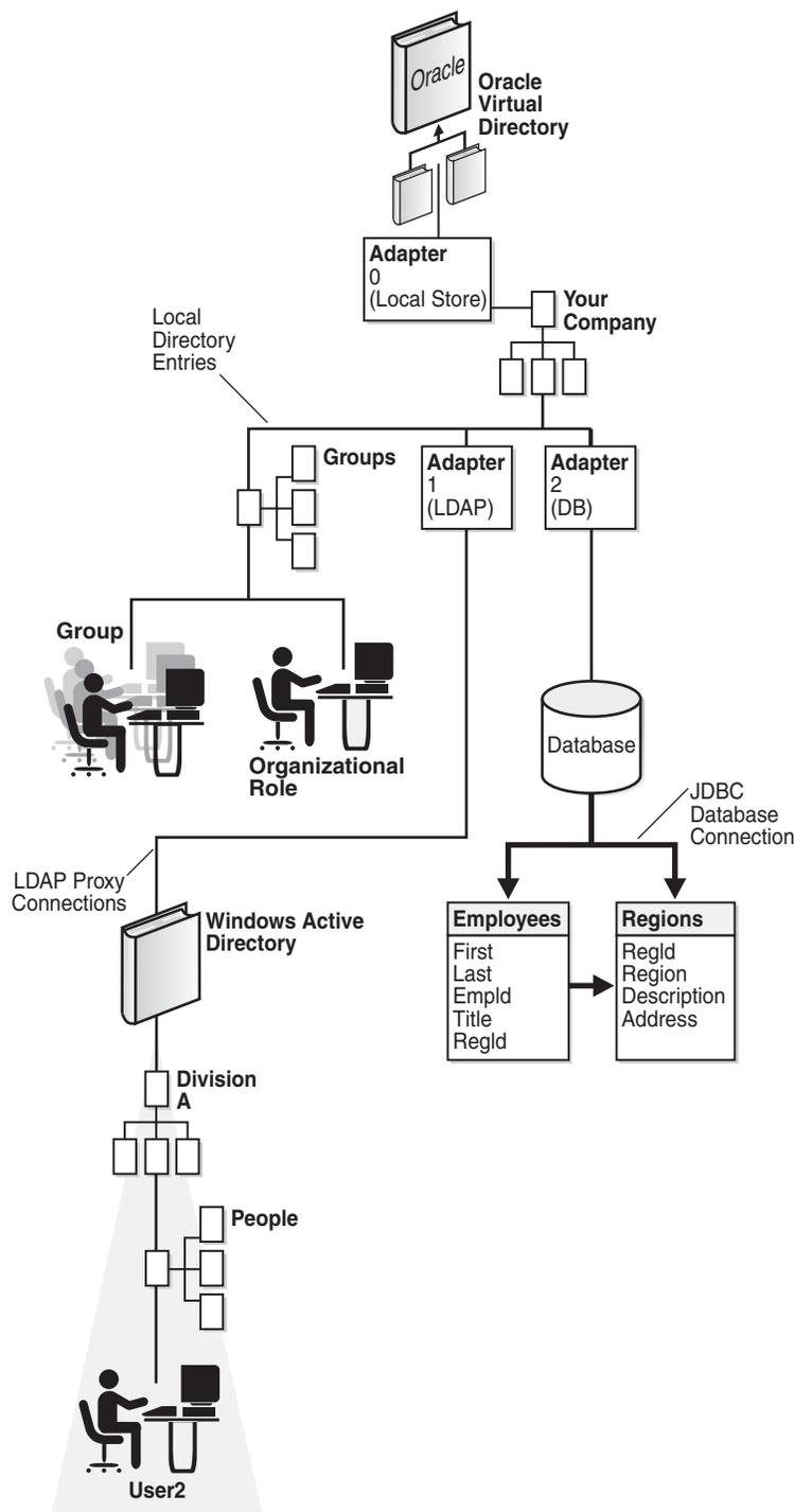
As shown in [Figure 2-5](#), Oracle Virtual Directory and its adapters allow different portions of the directory tree to be sourced from different repositories. In planning your virtual directory information tree structure, be sure you do not have two adapter roots that occupy the same root node. However, you may have an adapter appear to be a child node of another adapter.
