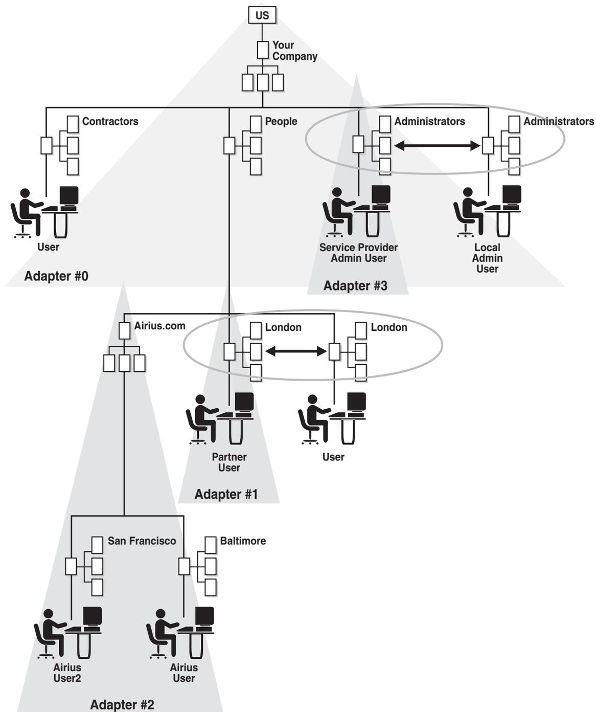
Traditionally, the overlapped directory structure would be unacceptable, however, Oracle Virtual Directory supports routing filters that control how it handles operations to overlapping namespaces.
