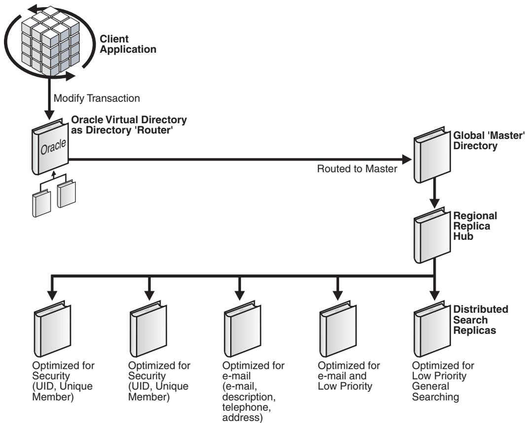
In Figure 1-5, the indexing strategy has been adjusted to create Class-of-Service replicas enabling replication to scale. Each class-of-service defines a set of directory replicas designed for specific application clients.
