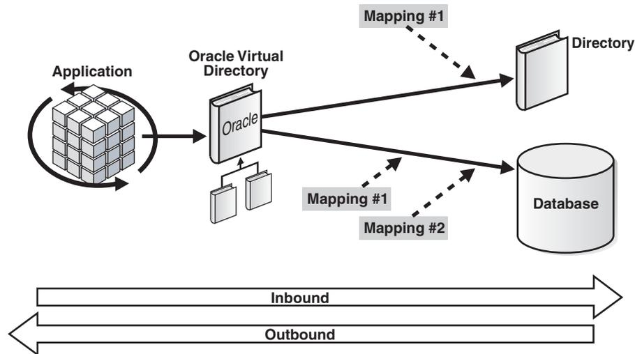
Each Mapping has an inbound and outbound flow, allowing it to translate one way as a request is received and reverse that translation as results are returned to the requesting application. This programmatic reversal is important because it is not usually possible for the server to guess intent.
