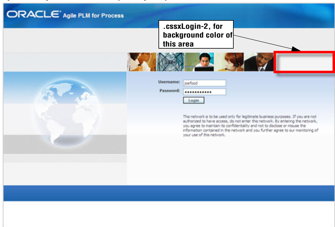
Figure 2-27: Login screen area affected by cssxLogin-2 style element of Brand.css
