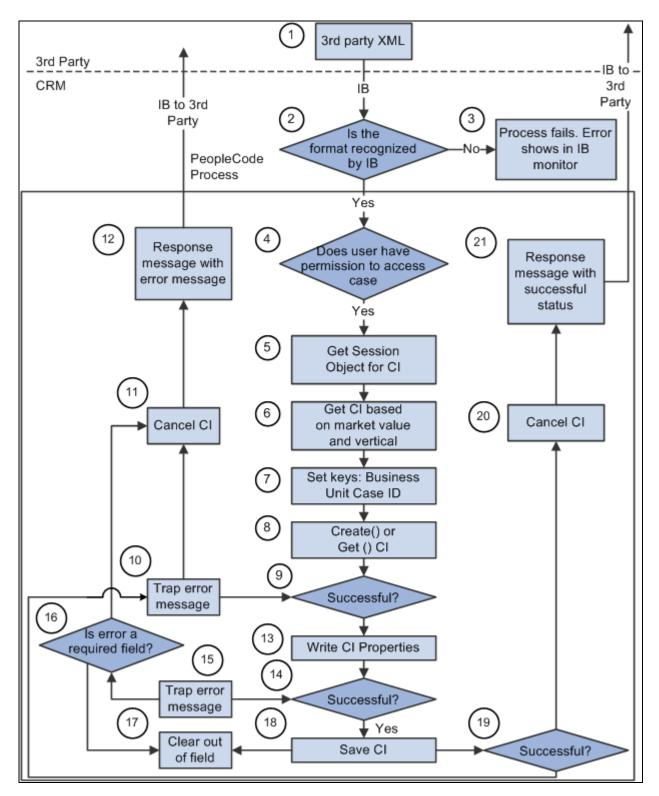
Process flow for EIP #1 and EIP #2
