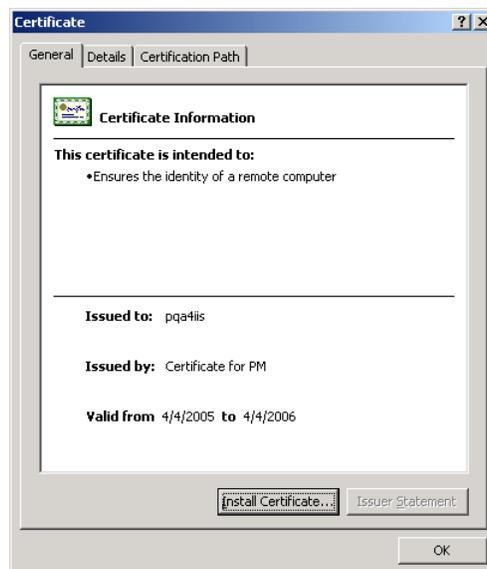
14. This certificate must now be installed into IIS. Open IIS and locate the Web site where ESSO-PG is installed. Right-click the Web site and click **Properties**.
