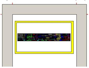
In this example a view has been superimposed on top of a yellow rectangle.
