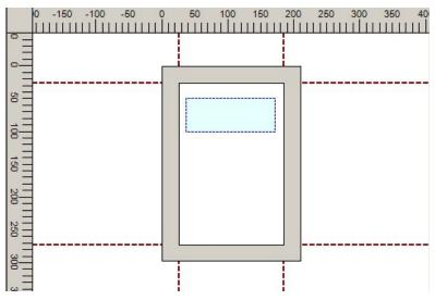
To add an image, move the cursor to the required start position in the Report Layout Designer. Hold down the left mouse button and drag to form a rectangle. When the left hand mouse button is released, the Select Data Source dialogue box will appear.
