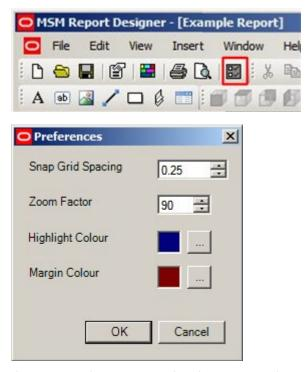
The Snap Grid spacing can then be set using the spin controls.
