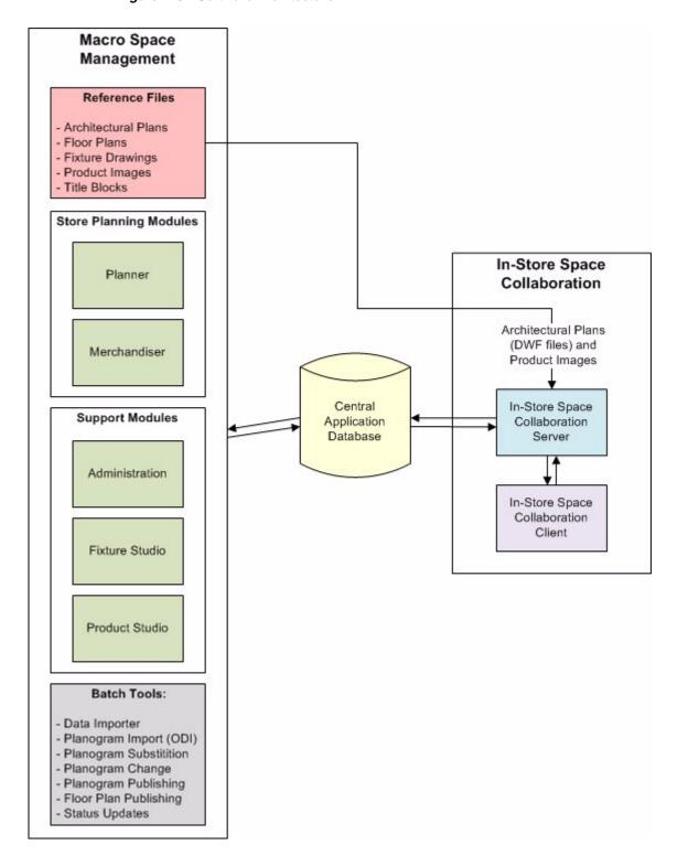
Figure 1-3 Software Architecture
