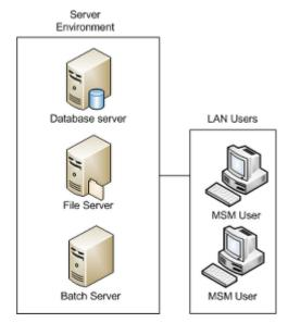
Figure 1–1 Typical Infrastructure with MSM Only Installed
