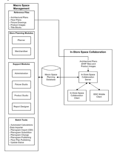
Figure 1-3 Software Architecture
