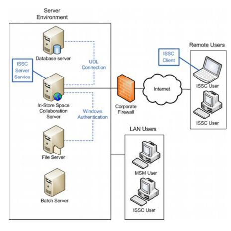
Figure 10-10 Connection Details for ISSC Server Service
