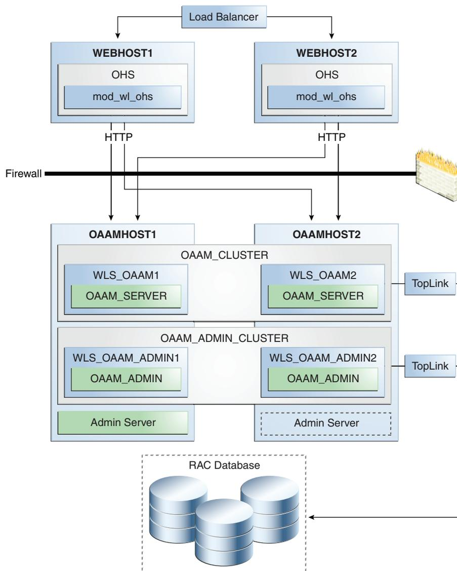
In [Figure 8–17](#), incoming requests are received by the hardware load balancer, which routes them to WEBHOST1 or WEBHOST2 in the web tier. These hosts have Oracle HTTP Server installed. The Oracle HTTP Server then forwards requests on to the WebLogic managed servers on OAAMHOST1 and OAAMHOST2 using the WebLogic plugin mod\_wl\_ohs.
