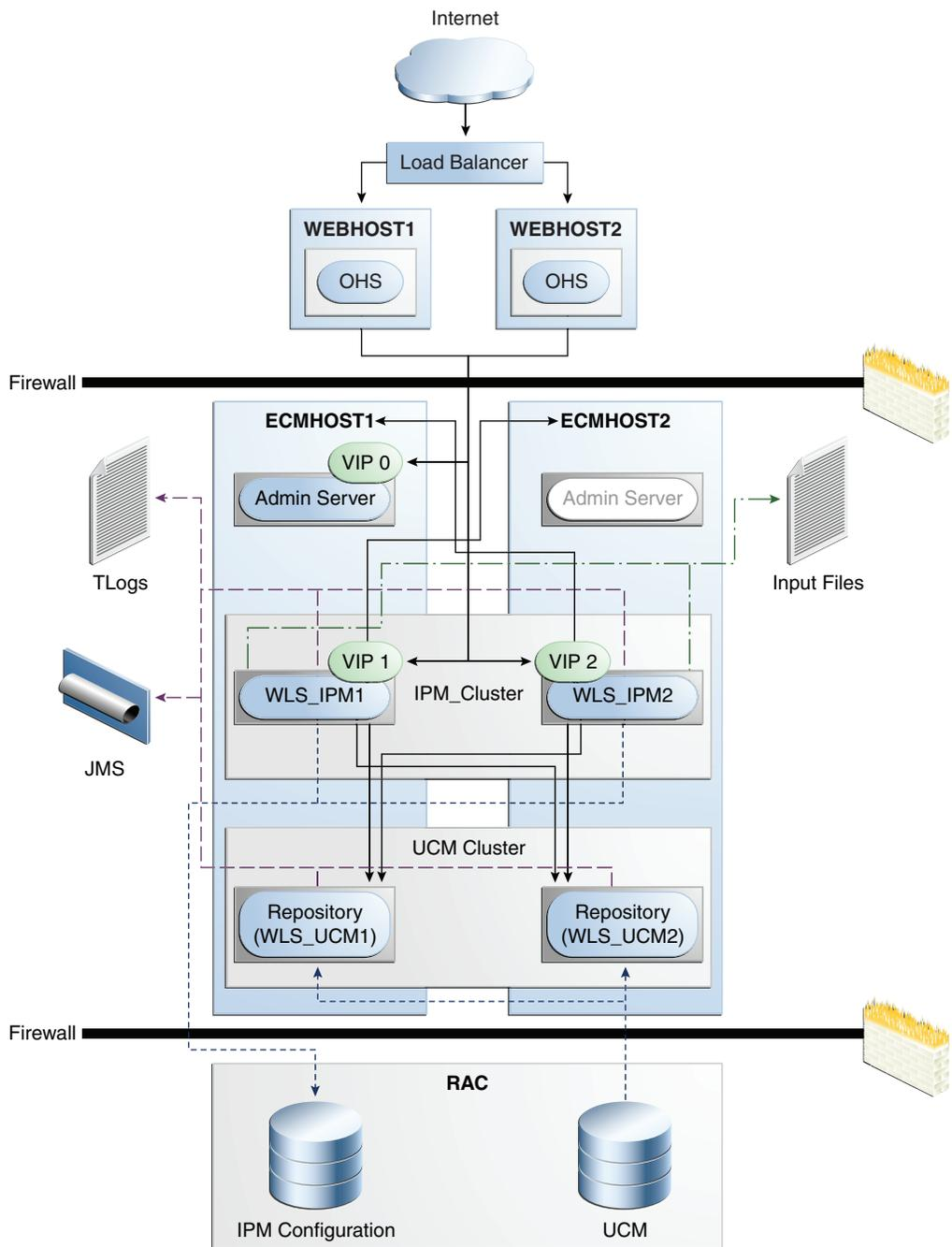
Oracle I/PM can be configured in a standard two node active-active high availability configuration. Although Oracle I/PM's UI layer will not fail over between active servers, its other background processes will.
