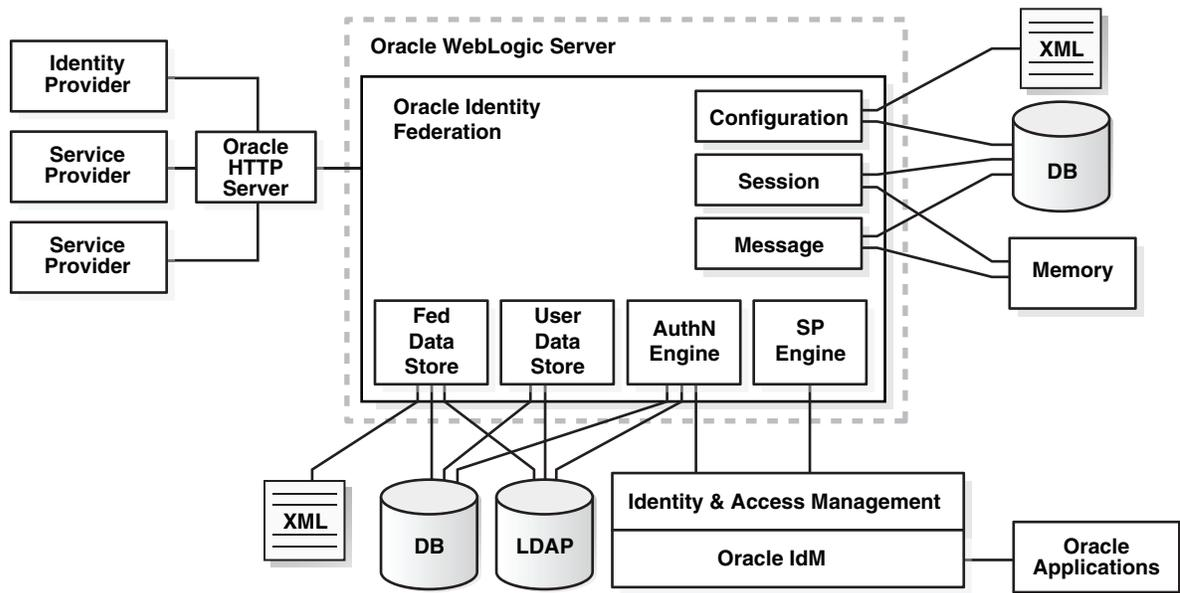
Figure 8–18 shows Oracle Identity Federation deployed on Oracle WebLogic Server in a non-high availability architecture and its relationship to other federation components.
