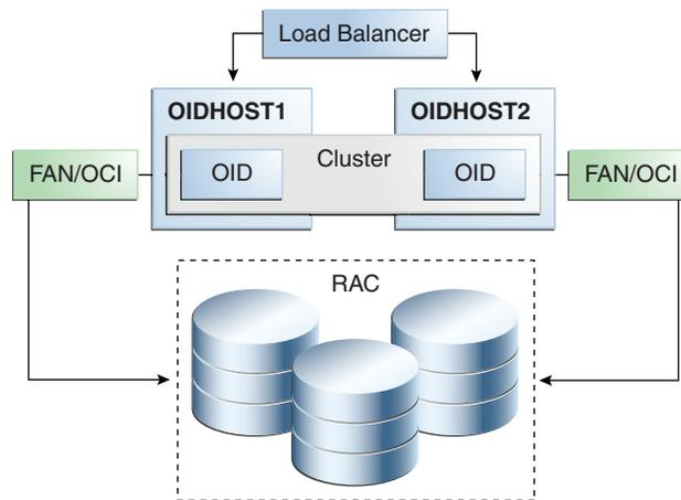
Figure 8–3 shows Oracle Internet Directory in the directory tier in a Cluster Configuration high availability architecture. Clustering is set up at installation time. The load balancing router routes LDAP client requests to the two Oracle Internet Directory instances that are clustered on OIDHOST1 and OIDHOST2.
