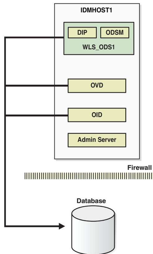
All the components in Figure 8–10 are deployed on the same host, but have separate Oracle homes and Oracle instances. Oracle Internet Directory uses a standalone Oracle database as the security metadata repository.
