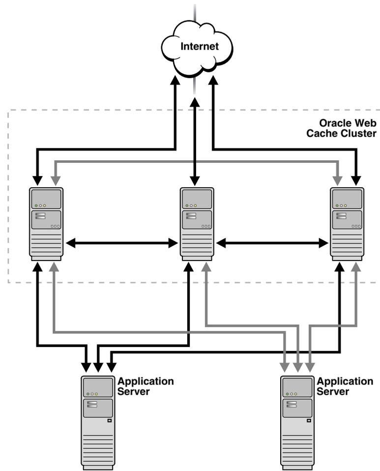
Oracle Web Cache uses the relative capacity of each cache instance to distribute the cached content among the cache cluster members. In effect, it assigns a cache cluster member to be the owner of a particular object. This content is called *owned content*.
