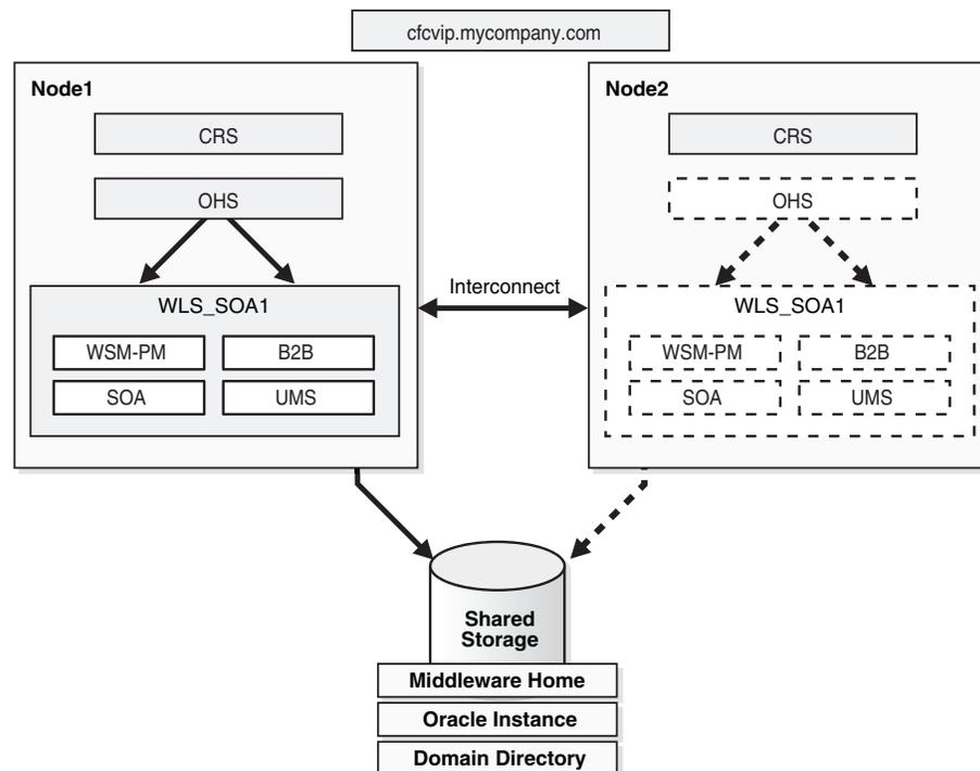
Figure 13–1 illustrates the CRS Example 1 topology. In this example, Oracle HTTP Server and SOA are installed in a two-node cluster. Oracle HTTP Server is managed by OPMN. The SOA installation has a WebLogic server running that it hosts four Java EE applications.
