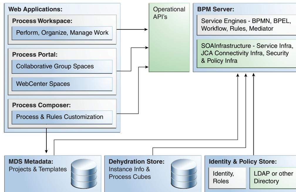
The web applications are stateless. The state is maintained in the Dehydration Service and the data is exposed through the Operational APIs or in MDS.
