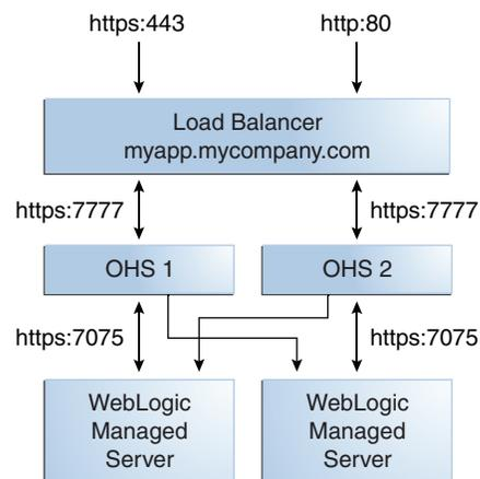
Figure 11–2 also shows how Oracle HTTP Server distribute requests to Web Logic Managed Servers. For High Availability, it is assumed that each pair of components (Oracle HTTP Server and Web Logic Managed Servers) exist on different hosts.
