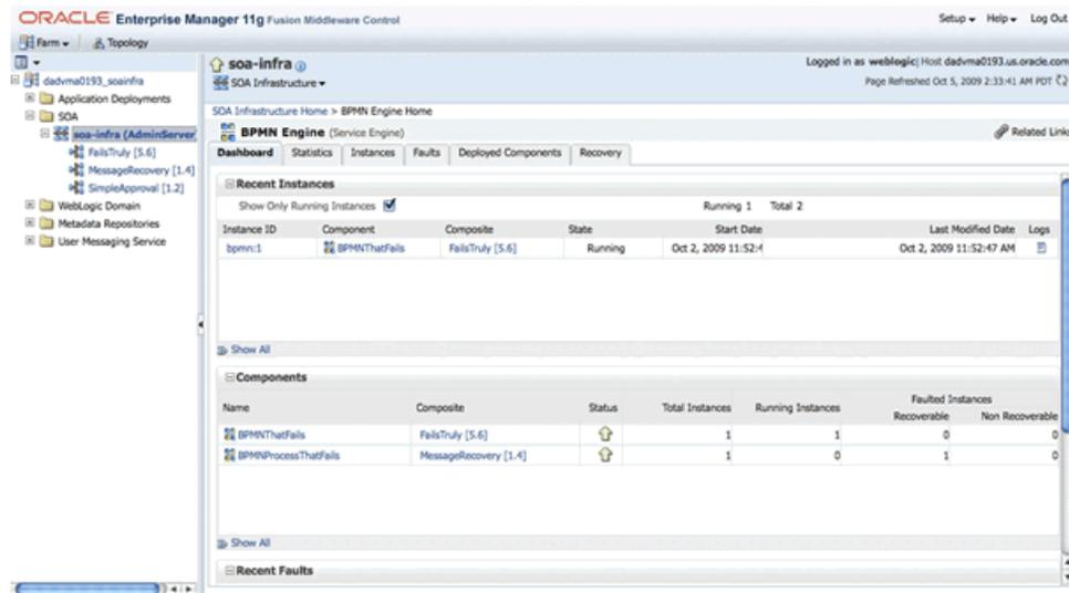
The home page of the BPMN service engine is comprised of several sub pages. The Dashboard page is the default page. For the recovery of BPMN service instances, select the Recovery tab, which opens the BPMN Service Engine Recovery page shown in [Figure 5–21](#).
