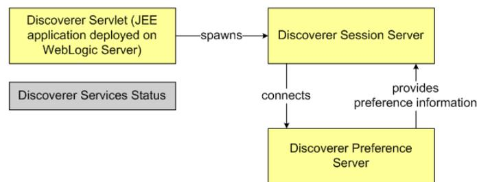
The **Discoverer Servlet** is a Java EE application that is deployed on a managed server, which can be started and shutdown through the Oracle WebLogic Server administration console and by using the Oracle Enterprise Manager Fusion Middleware Control. The Discoverer Servlet is a stateless process.
