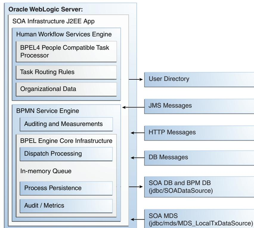
The BPMN service engine leverages the BPEL PM dispatcher module to dispatch incoming messages from binding components (JMS, database, Web Services) for processing.
