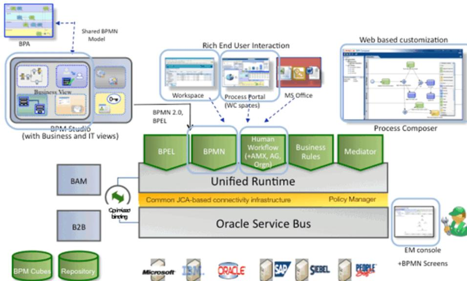
A SOA composite application is the basic unit of deployment to the SOA runtime. Service components (BPEL process, business rule, human task, and Mediator routing rule) are the building blocks of a SOA composite. Components are targeted to service engines during deployment while services and references are enabled using the binding components. At runtime, messages are received by the binding component and are then routed to the appropriate service engine(s) by the Service Infrastructure.
