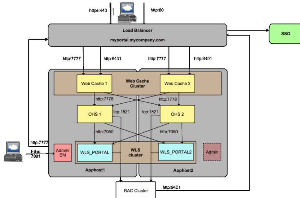
The Oracle Portal high availability setup includes two or more Oracle Web Cache instances. These Oracle Web Cache instances are clustered together to provide cache consistency and failover. Each Oracle Web Cache is configured to route traffic to two or more Oracle HTTP servers, and these servers load balance incoming requests.
