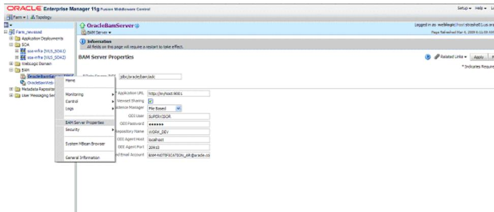
The properties exposed by Oracle Enterprise Manager are a mix of the information contained in two different files: `BAMServerConfig.xml` and
