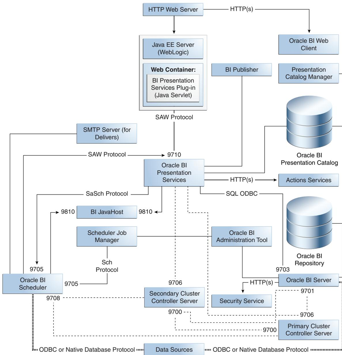
Note that the port numbers shown in [Figure 15-1](#) are the default port numbers for a simple installation with one component of each component type on a single machine. When you use Oracle Enterprise Manager Fusion Middleware Control, you can choose a port number range and Enterprise Manager will assign the port numbers.
