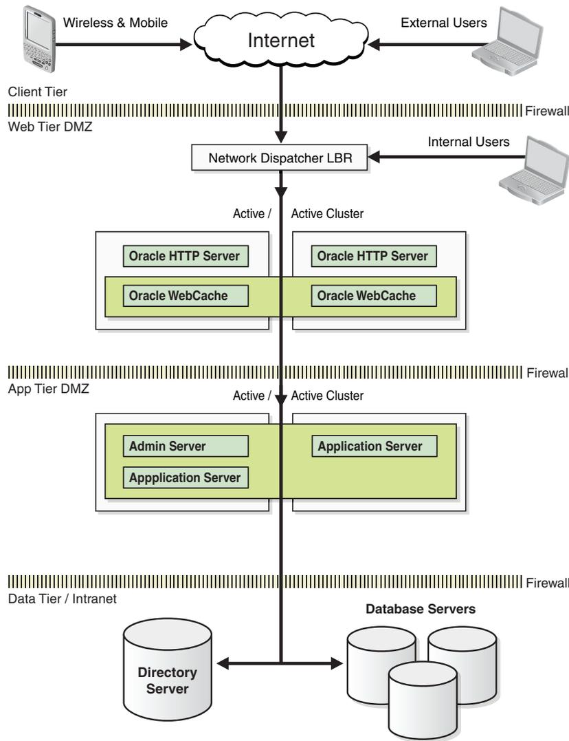
As shown in Figure 2-3, this topology represents a multi-tiered architecture. Users access the system from the client tier. Requests go through a hardware load balancer,
