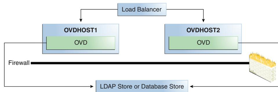
[Figure 8–5](#) shows Oracle Virtual Directory in the directory tier in a high availability architecture. The two-node cluster is set up at installation time. The load balancing router routes requests to the two Oracle Virtual Directory instances that are clustered on OVDHOST1 and OVDHOST2. Fast Connection Failover (FCF) is used for notification when an Oracle RAC instance becomes unavailable.
