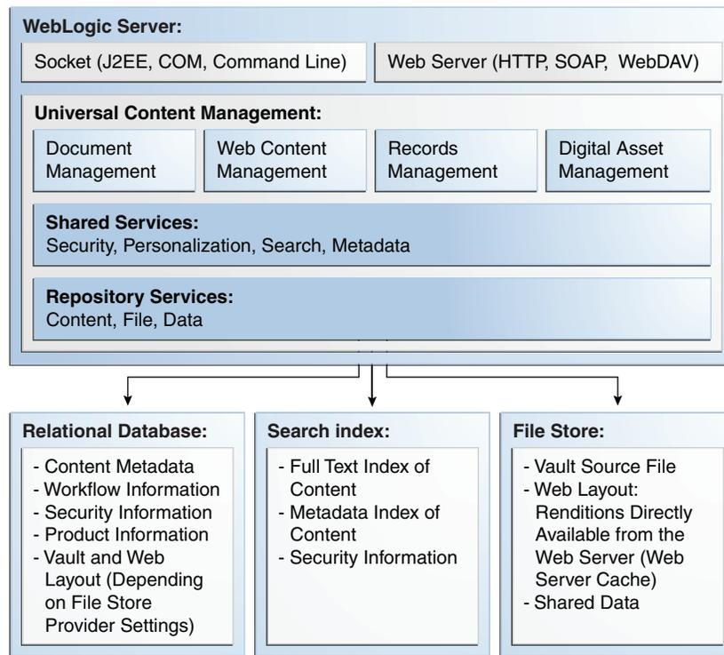
An instance of Oracle UCM runs within an Oracle WebLogic Managed Server environment. WebLogic Server is responsible for the lifecycle of the Oracle UCM application, such as starting and stopping the application. WebLogic Server is
