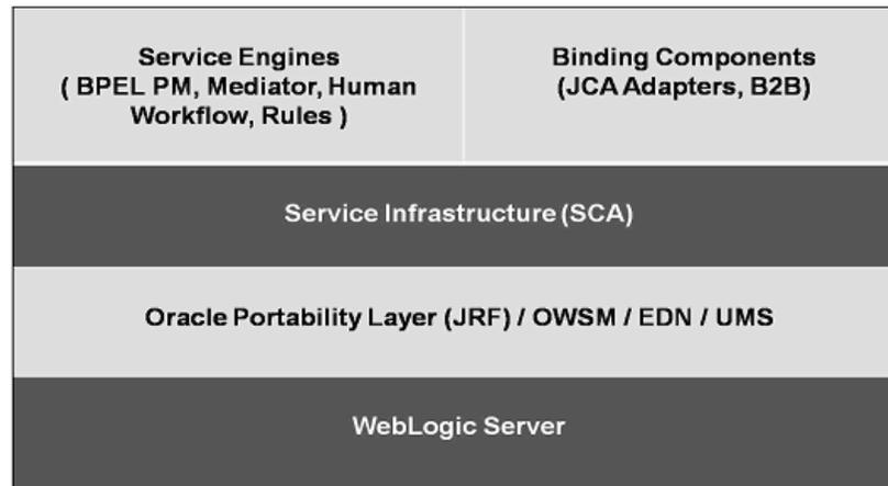
The SOA runtime executes within the context of an application server such as the Oracle WebLogic Application Server. It leverages the underlying application server capabilities for load balancing and high availability.
