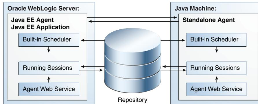
Oracle Data Integrator run-time agents manage integration processes. Oracle Data Integrator agents are components that run the integration jobs deployed in a production configuration as scenarios stored in a repository.
