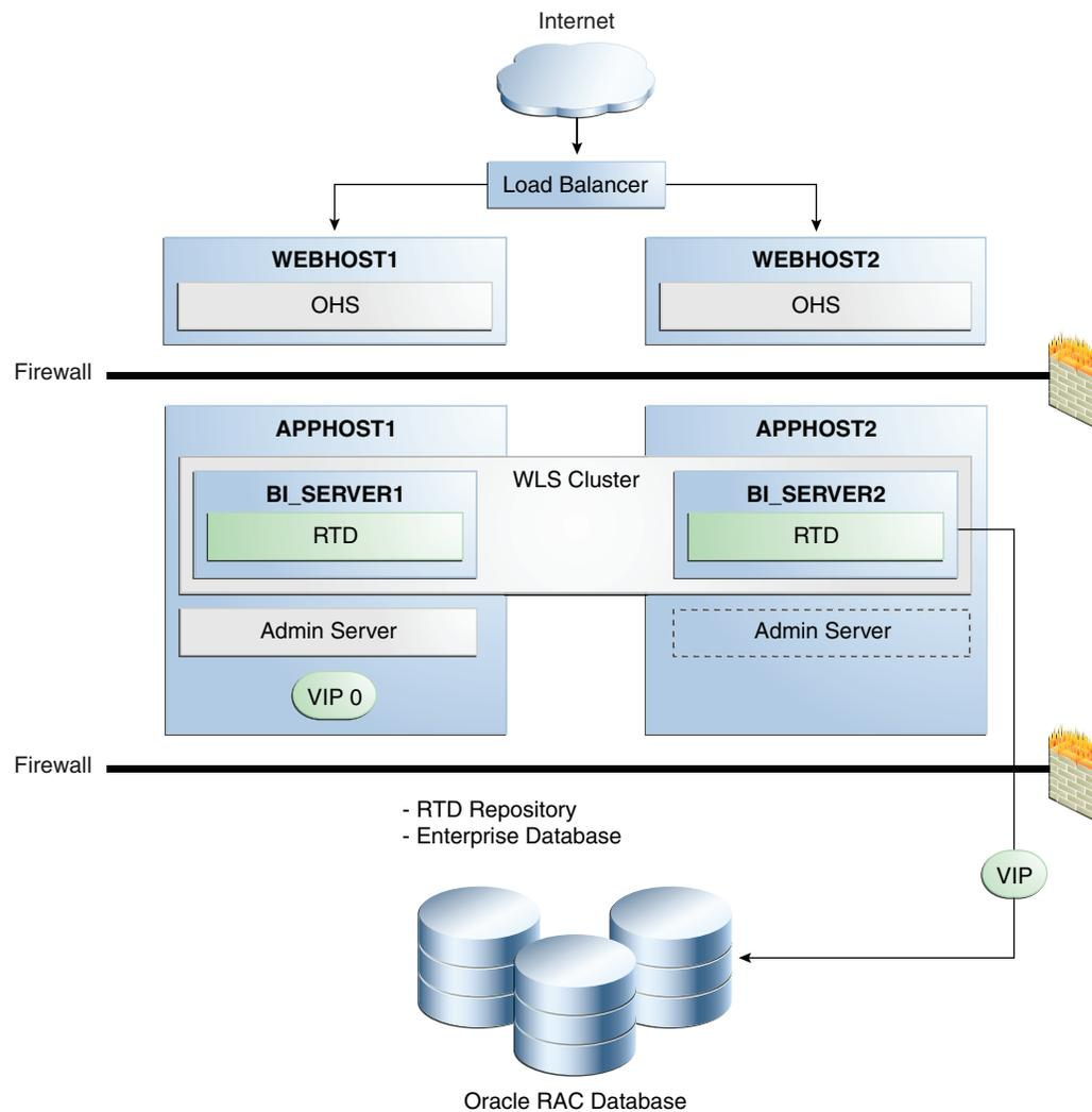
In Figure 15–10, incoming requests are received by the hardware load balancer, which routes them to WEBHOST1 or WEBHOST2 in the web tier. These hosts have Oracle HTTP Server installed.
