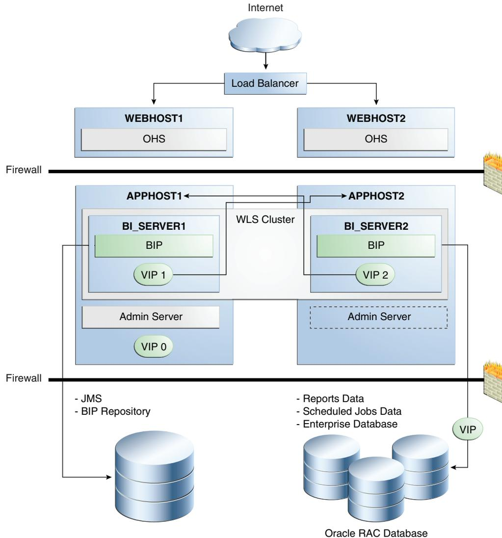
In Figure 15–8, incoming requests are received by the hardware load balancer, which routes them to WEBHOST1 or WEBHOST2 in the web tier. These hosts have Oracle HTTP Server installed.
