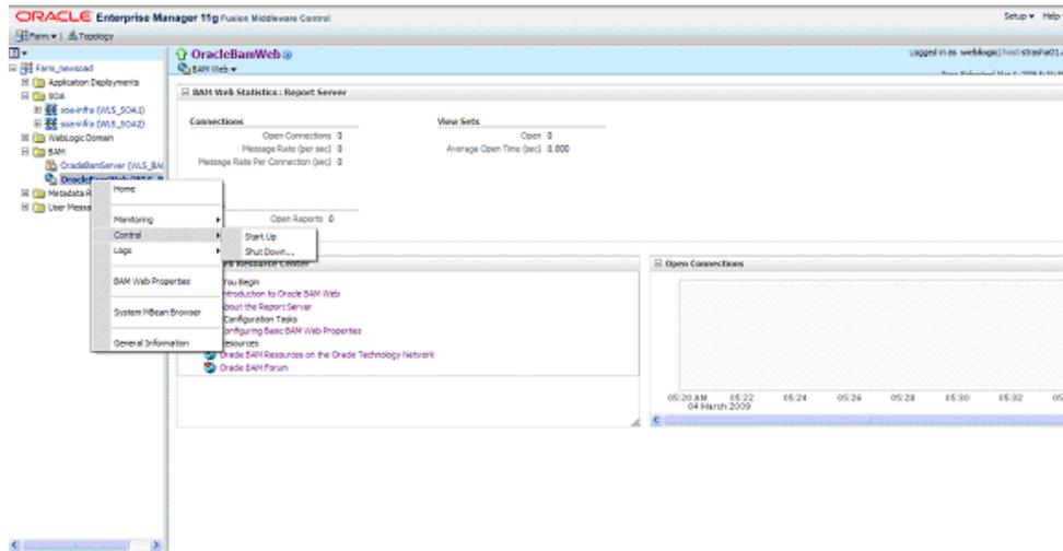
**Note:** Although Enterprise Manager offers separate start and stop for Oracle BAM Server and Oracle BAM Web Applications, this is in reality a stop operations that affects both components, meaning if Oracle BAM Server is stopped from Enterprise Manager, the corresponding Oracle BAM Web Applications are also stopped, and the reverse is also true. This also applies for start operations.
