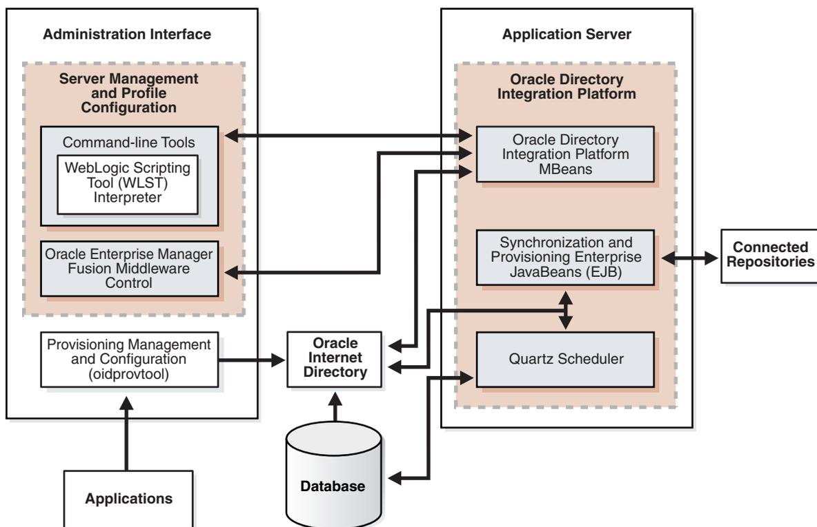
Figure 8–6 shows the various components of Oracle Directory Integration Platform. Oracle Internet Directory is synchronized with connected directories using Oracle Directory Integration Platform's Synchronization Enterprise JavaBeans (EJB) and the Quartz Scheduler.
