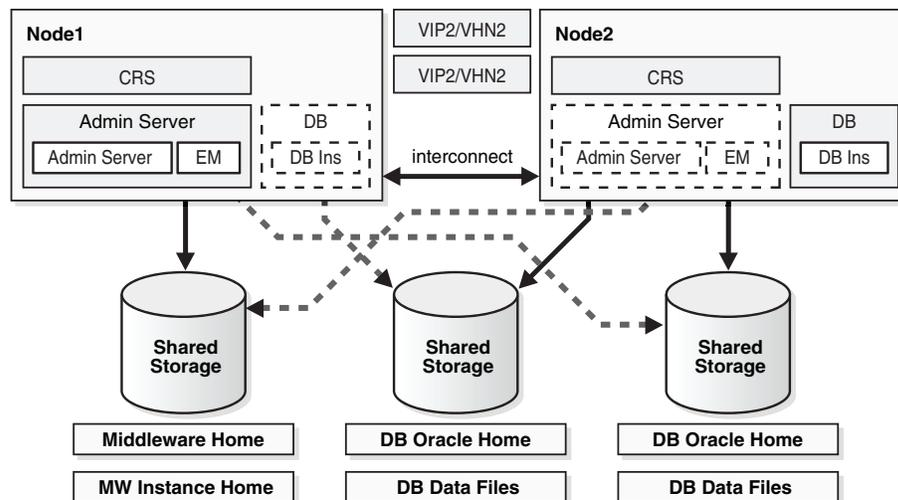
Figure 13–2 illustrates the CRS Example 2 topology. In this example topology, WebLogic Server and the Oracle database are installed on a two-node cluster with the following characteristics:
