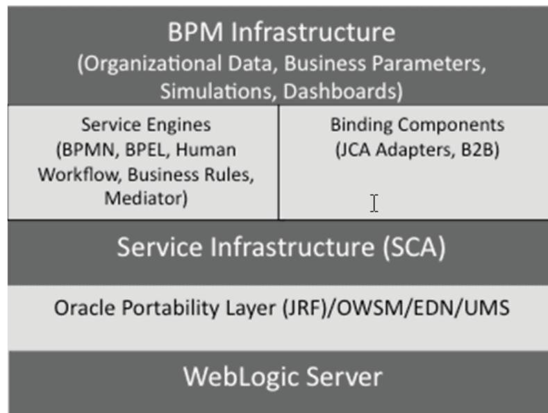
The BPM runtime executes within the context of an application server such as the Oracle WebLogic Server. It leverages the underlying application server capabilities for load balancing and high availability.
