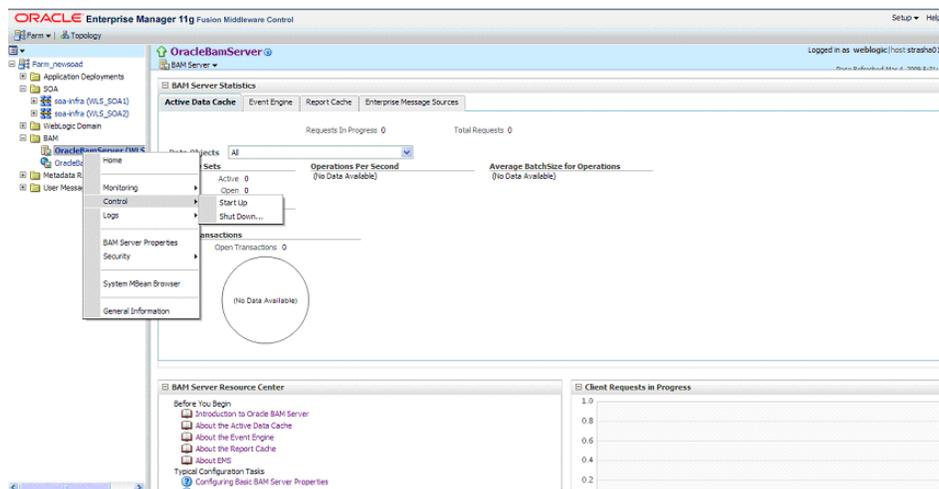
The BAM Web Applications run collocated by default in the same managed server as BAM Server. For example, the BAM server and BAM Web Applications are part of the same deployment in WebLogic Server Administration Console. They can't be stopped and managed separately from BAM Server by default. It is possible though, as explained in later sections, to manipulate WebLogic Server application targeting to
