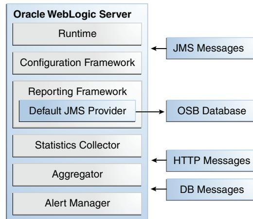
When Oracle Service Bus is deployed in a high availability configuration, the Aggregator and Alert Manager components are singletons that should be deployed only on one host in the cluster.
