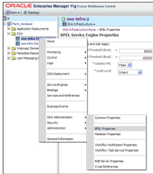
If you are using Oracle SOA Suite in a clustered environment, any configuration property changes you make in Oracle Enterprise Manager on one node must be made on all nodes. Configuration properties are set in Oracle Enterprise Manager through the following options of the SOA Infrastructure menu:
