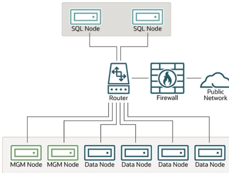
In this case, you can set the rules in the hardware firewall to deny any external traffic except to SQL nodes and API nodes, and then permit traffic to them only on the ports required by your application.
