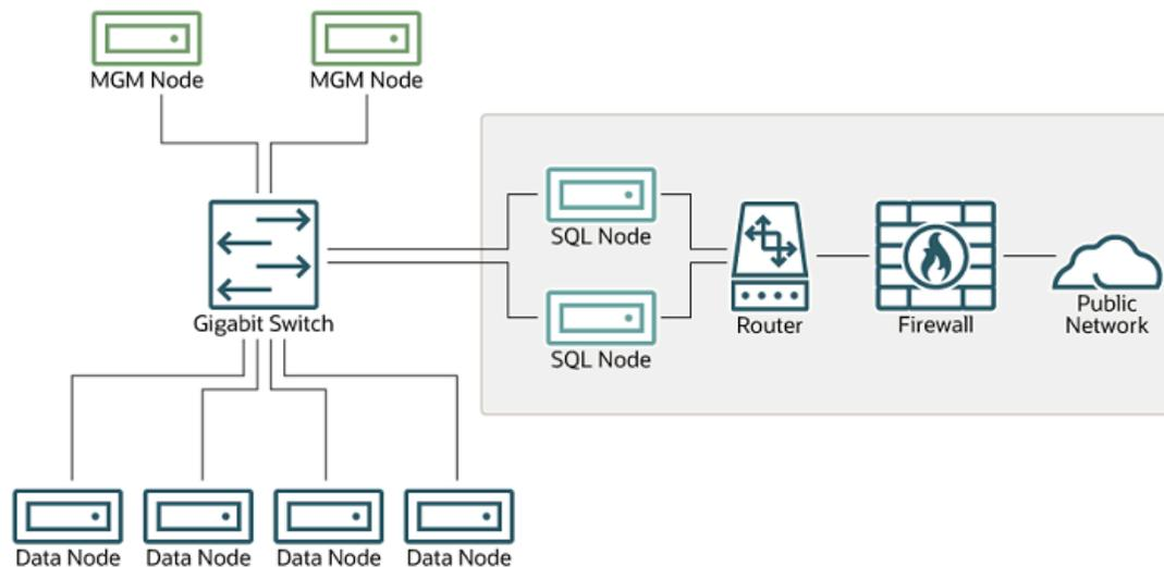
This setup has two networks, one private (solid box) for the Cluster management servers and data nodes, and one public (dotted box) where the SQL nodes reside. (We show the management and data nodes connected using a gigabit switch since this provides the best performance.) Both networks are protected from the outside by a hardware firewall, sometimes also known as a *network-based firewall*.
