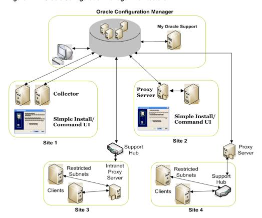
Figure 1–1 Oracle Configuration Manager Architecture
