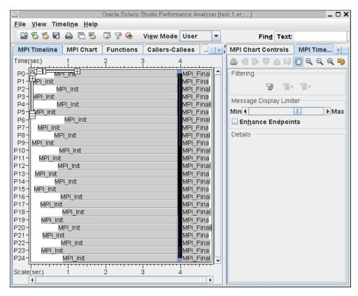
The experiment opens on the MPI Timeline tab. The MPI Chart tab is next to it. In the right panel you can see the MPI Chart Controls and MPI Timeline Controls tabs.
