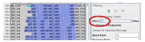
The Messages slider controls the number of message lines displayed on the screen. At Min, only functions are displayed in the MPI Timeline tab.
