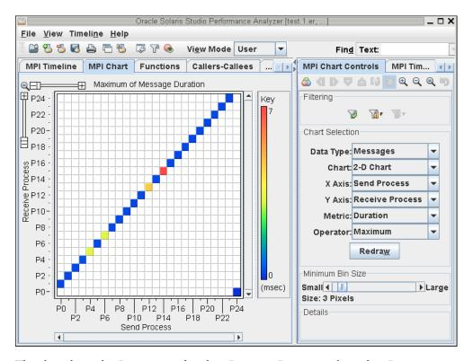
This chart shows that Process 0 sends only to Process 1. Process 1 only sends to Process 2, and so on. The color of each box is set by the metric selected (Duration) and the operator
