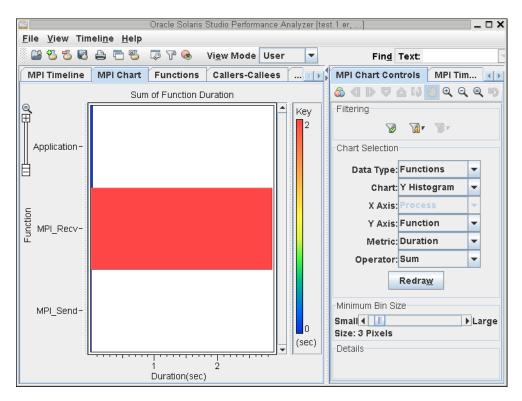
The MPI Chart tab opens with a chart that shows the sum of the durations of the functions as they ran in all the processes. The vertical rainbow scale to the right of the chart shows the mapping between colors and values. The MPI\_Send and Application functions take almost no time, whereas in the example, the cumulative time in MPI\_Recv was nearly three seconds.
