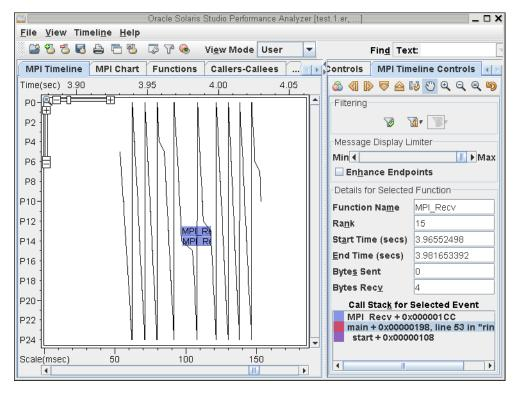
6. Click the Filter Undo and Redo buttons to toggle the context around the long duration functions.
