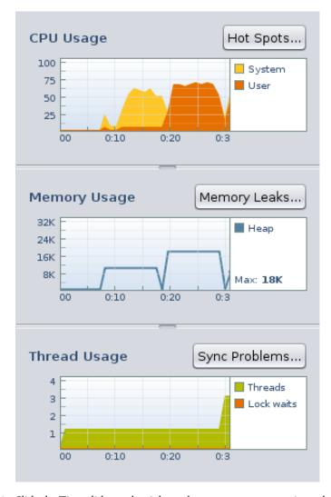
4. Slide the Time slider to the right so that you can see two points where the threads increase to three. The first increase in threads corresponds to the PARALLEL DEMO portion of the program run, where the main thread starts two additional threads to do the work of writing to a file and performing calculations, in parallel. otice that the memory usage and CPU usage are a bit higher during this portion, but thee two tasks are completed in much less time than in the SEQUENTIAL DEMO portion.
