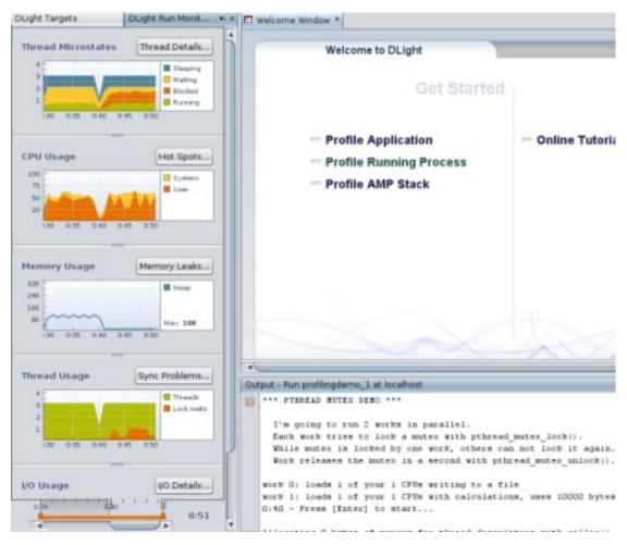
5. Click the Thread Details button to display details about the thread microstates. The Thread Details window opens to display a graphical timeline representation of all the threads run in the program along with detailed state information.
