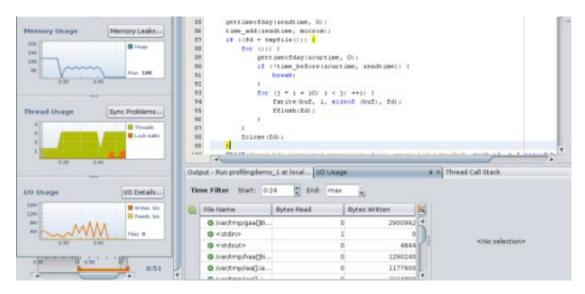
15. The I/O Usage details tab shows that multiple files are open during the PTHREAD MUTEX DEMO portion of the run. One thread is writing to a file, and every second it switches the file it writes to, as in the PARALLEL DEMO portion. However, because mutex locks are used, sometime the writing thread is blocked by the calculating thread and cannot continuously write to files.
