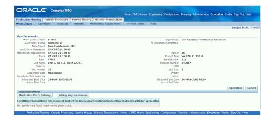
Enigma Integration displays buttons for viewing Wiring Diagram Manual (WDM) and Illustrated Parts Catalog (IPC) as applicable.
