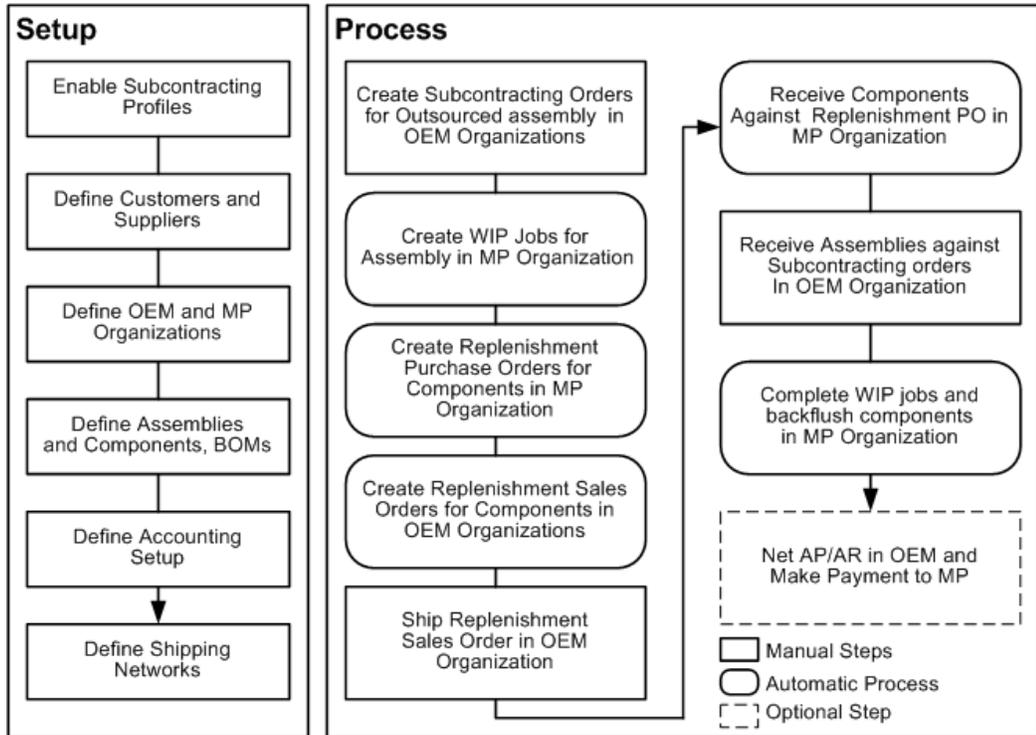
This diagram illustrates the setup and process flow for Full Outsourcing:
