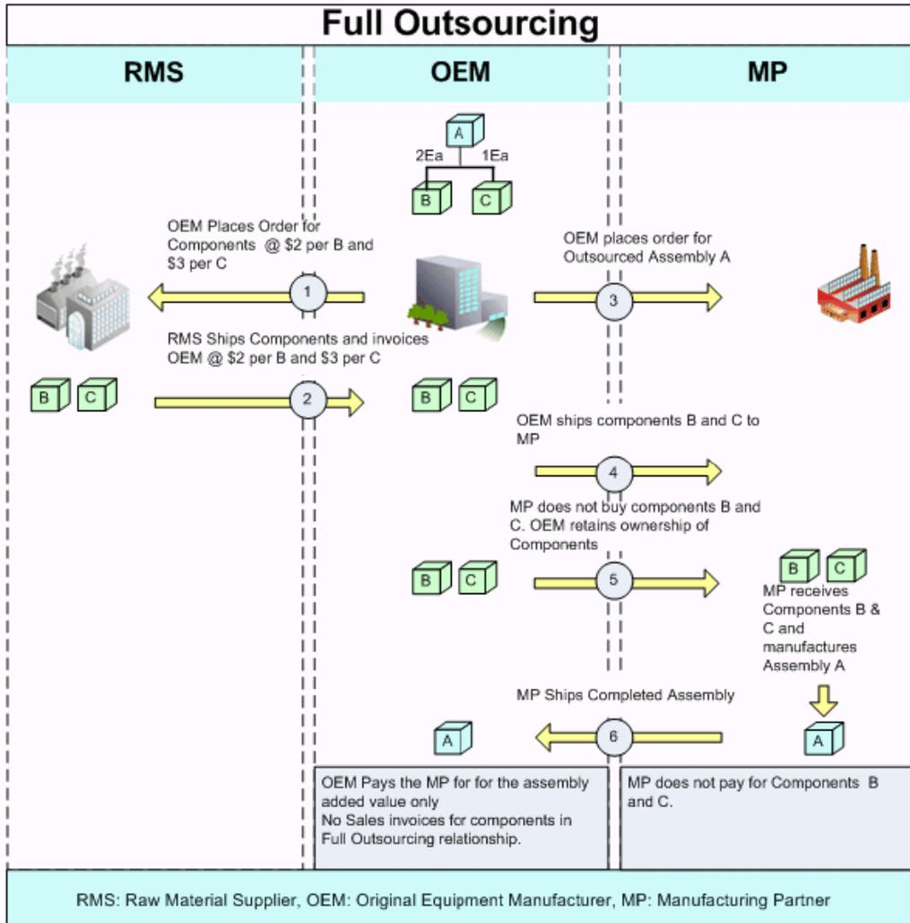
The Full Outsourcing Process diagram describes a full outsourcing business flow , where the OEM outsources Assembly A to an MP, buys components from the RMS and ships the components to the MP to manufacture A at the MP's premises while retaining ownership of components B and C:
