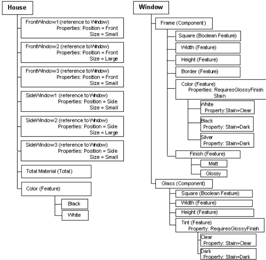
Example House Model, page 3-2 shows the Model House as the parent Model, and a Model called Window is its child (referenced) Model. The Window Model contains a Frame Component and a Glass Component, and both Components have various types of Feature nodes.
