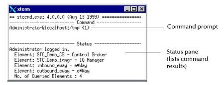
On UNIX systems, the **stccmd** utility uses a two-pane display. The top pane provides the command prompt; the bottom displays the command results.
