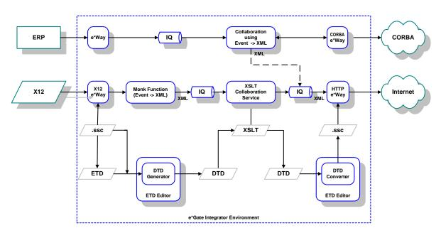
Figure 14 XML Toolkit Components in Sample Configuration
