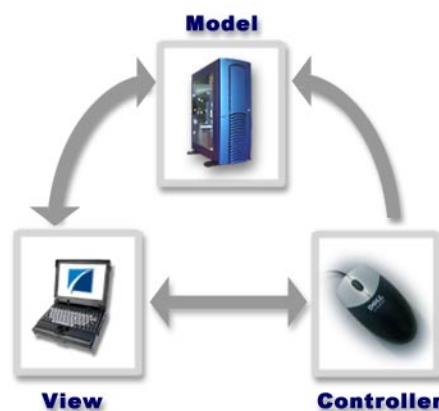
Figure 2 Model/View/Controller (MVC) Architecture
