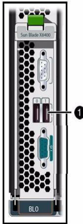
**Figure Legend** Server Module Front Panel USB Ports
