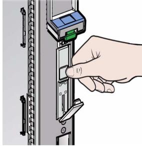
4. Holding the opened ejector lever, pull the ejector lever toward you and slide the filler panel from the HDD slot.
