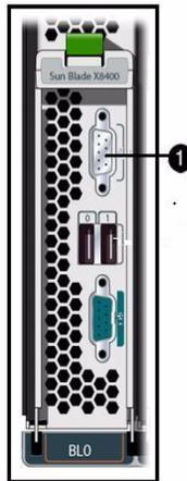
**Figure Legend** Server Module Front Panel VGA Port
