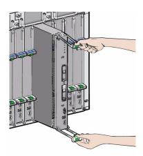
3. Slide the server module into the vacant server module chassis slot.
