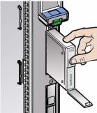
7. Ensure that the HDD ejector lever is two-thirds open (approximately 60 degrees with respect to the faceplate) when sliding in the HDD into the slot.
