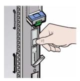
4. Holding the opened ejector lever, pull the ejector lever toward you and slide the filler panel from the HDD slot.
