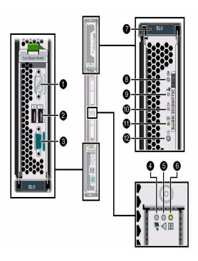
Figure Legend Server Module Indicators and Buttons
