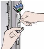
8. Using your thumb or finger, press on the middle of the HDD front faceplate until the ejector lever engages with the server module.
