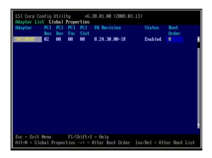
3. With the LSI 1068E adapter highlighted in the first screen, press Enter. The main screen of the utility opens.
