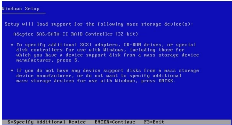
FIGURE 6-6 Example Specify Additional Device Screen With Sun Blade RAID 5 Expansion Module Selected
