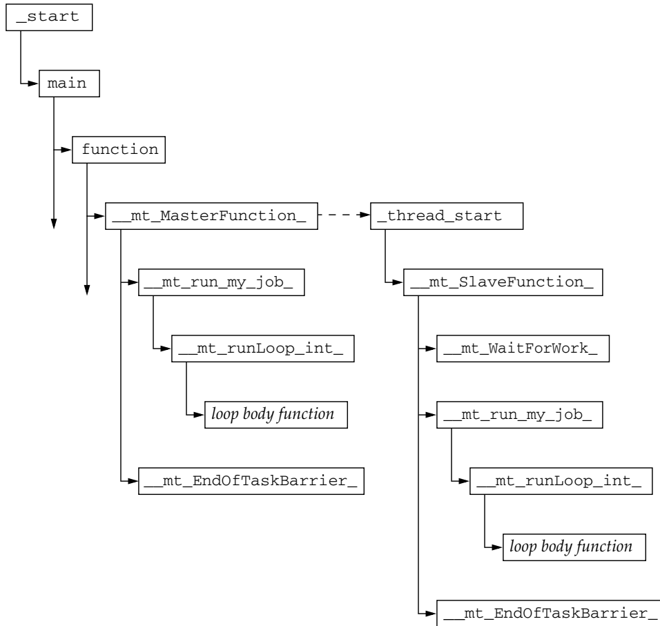
FIGURE 5-1 Schematic Call Tree for a Multithreaded Program That Contains a Parallel Do or Parallel For Construct
