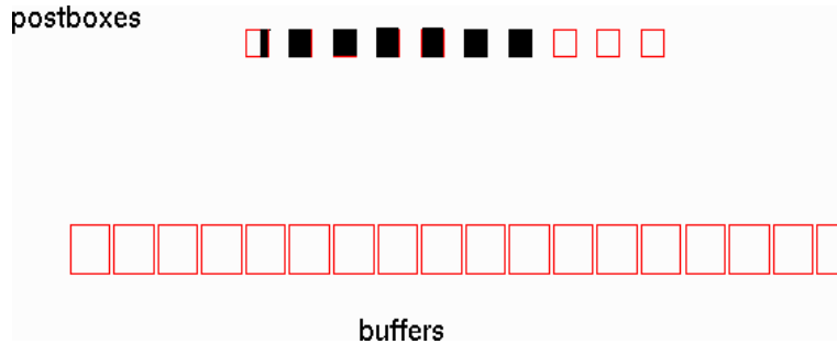
FIGURE B-14 A short RSM message. Message data is buffered in the shaded areas.
