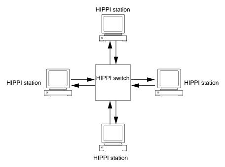
FIGURE 6-4 HIPPI Network Configuration Using a Switch
