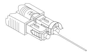
FIGURE 2-3 Cleaning the End of a Fiber-Optic Cable
