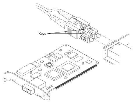
FIGURE 2-2 Aligning SC Type Fiber-Optic Cable Connectors
