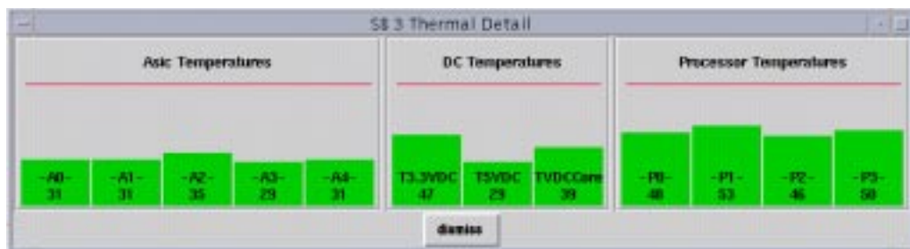
FIGURE 6-3 System Board Thermal Detail
